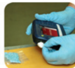
Analyze through sealed packaging for most samples.
